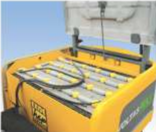
48V battery & AC traction for longer hours of operation
