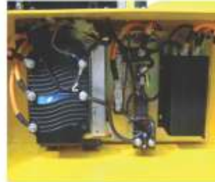
Side mounted controller for easy maintenance
