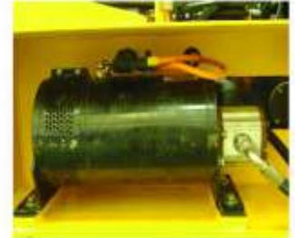
Side mounted hoist motor for easy maintenance
